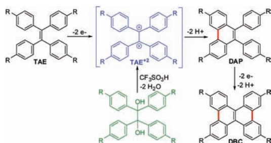
Scheme 1. Sequential Oxidative Transformation of TAE to DAP and DBC
